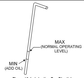
Figure 16. Lubrication Box Dipstick
